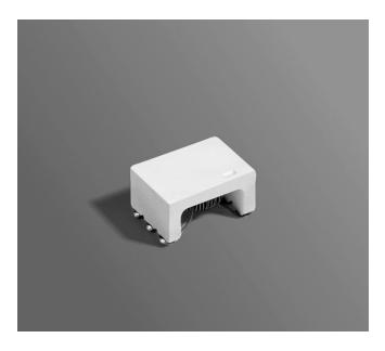
This low cost transformer is designed for up to 300 kHz and above to sense continuous currents up to 3 Amps. The current windings can be connected in series to provide twice the output sensitivity. It offers 500 Vrms interwinding isolation.
