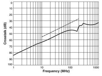
802.3af specification: 45 dB min at 30 MHz 40 dB min at 60 MHz 33 dB min at 100 MHz
