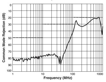
802.3af specification: 50 dB min from 1 MHz to 10 MHz 30 dB min from 10 MHz to 125 MHz 20 dB min from 125 MHz to 500 MHz
