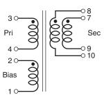
Secondary windings to be connected in parallel on the PC board
