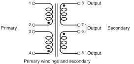
windings to be connected in series on the PC board.
