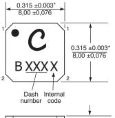
\* Dimensions are of the case not including the termination. For maximum overall dimensions including the termination, add 0.005 in / 0,13 mm.
