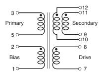
The secondary windings are to be connected in parallel on the PC board.
