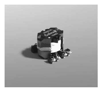
This surface mount flyback transformer is designed for use with Texas Instruments LM5000 DC/DC regulator. The core completely encloses the windings to minimize EMI interference. The transformer features very low DCR, 500 Vrms isolation and a leakage inductance rating of just 1.0  $\mu$ H. Coilcraft can also custom engineer a transformer to meet your specific requirements.
