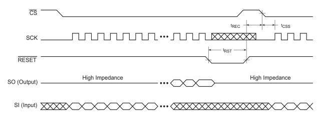
Note: 1. The  $\overline{CS}$  signal should be in the high state before the  $\overline{RESET}$  signal is deasserted.
