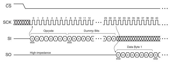
Figure 25-11.Read Security Register (Opcode 77h)
