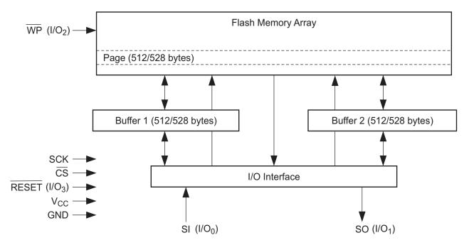
Note: I/O<sub>3-0</sub> pin naming convention is used for Dual-I/O and Quad-I/O commands.
