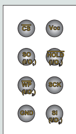
Figure 1-3. 8-ball WLCSP (Bottom View)
