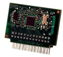
The CPM 5000 decreases product time-to-market for LonWorks® based devices. It includes all the components needed to implement a control node using the FT 5000 Smart Transceiver — the smallest, fastest, highest performance, lowest cost twisted pair LONWORKS transceiver on the market.
