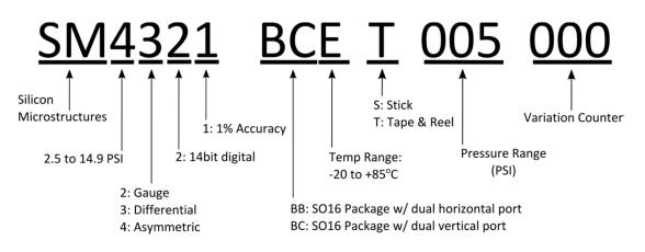
\*Custom calibration pressures and voltages are available to meet specific customer demands. Dual vertical or dual horizontal ports available.
