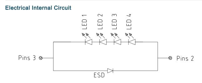
Pins 1a: NTC/Substrate potential, isolated from Cathode and Anode Pins 1b: NTC Pins 2: Anode Pins 3: Cathode
