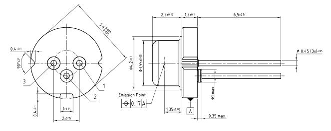
Pin 1: LD Anode Pin 2: LD Cathode, PD Anode (case) Pin 3: PD Cathode
