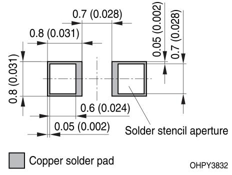
For superior solder joint connectivity results we recommend soldering under standard nitrogen atmosphere.
