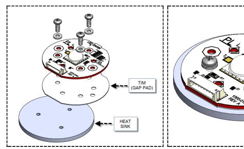
Mounting structure (exploded view)
