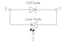
Pin 1: LD Anode Pin 2: Case Pin 3: LD cathode
