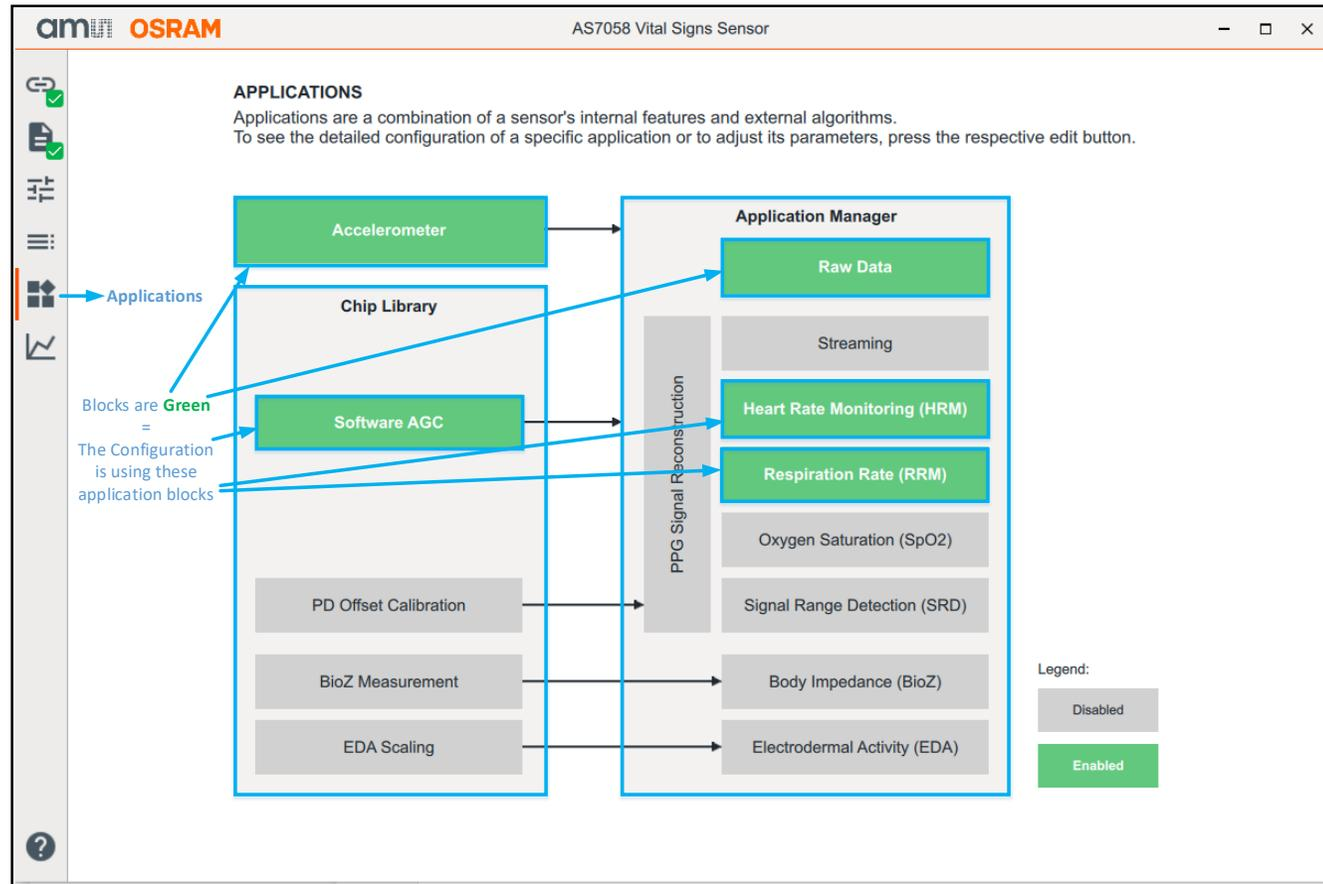
Fig. 10: Overview of the GUI - Applications
