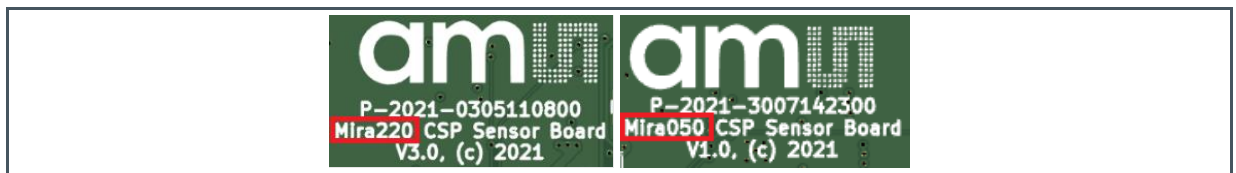
Figure 7: Mira Sensor Board Types Printed on the PCB.
