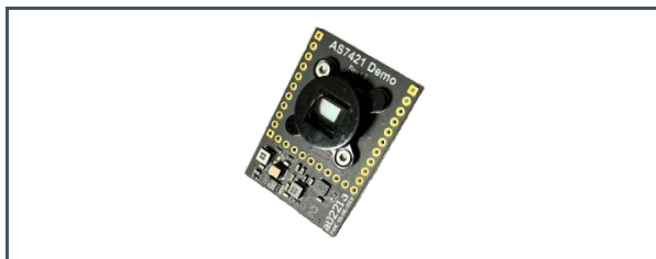
Figure 5: Top view of the AS7421 sensor board
