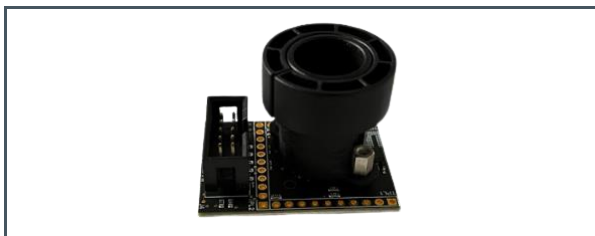
Figure 6: Bottom view of the AS7421 sensor board with the mounting holder
