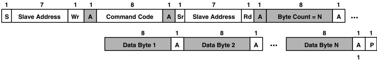
Figure 21. SMBus Block Read or I 2 C Read (Combined Format) Protocols
