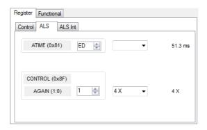
ATIME Register (0x81) controls the ALS integration time. The actual time is: (256-ATIME) \* 2.7 mS
