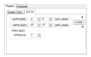
The AILTH (0x85) and AIHTH (0x87) values are 16 bit thresholds for the upper and lower trigger points. Each is set using two 8-bit registers.
