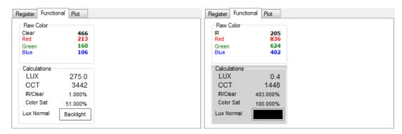
The Color photodiodes raw output values are shown. If the IR channel is selected, the top line of the Raw Color section will be replaced with the IR value as shown in the image on the right. While the IR data is selected, the Calculated fields are all invalid (since the first input channel is not the Clear photodiode), so the Calculations section is shown with a gray background to remind the user that the values are incorrect.
