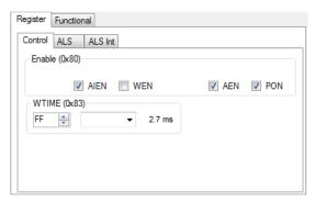
The Control sub-tab allows enabling and disabling functionality of the part and also controls the wait time multiplier (WTIME).
