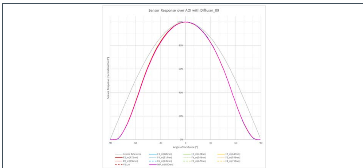
Figure 18: Angle Dependence Of Kimoto OptSaver L-57 For Spectral Scanning
