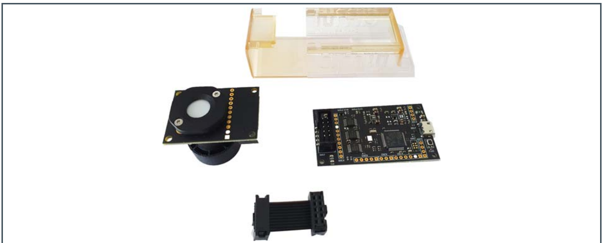
Figure 7: Sensor And Tiny Board, Direct Plugged With USB-Interface, Insert-able In Plastic Housing
