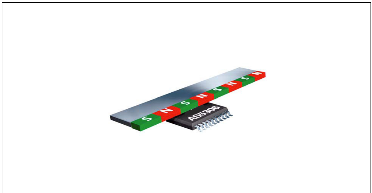
Figure 21: AS5306 (AS5304) with Magnetic Multi-Pole Strip Magnet for Linear Motion Measurement
