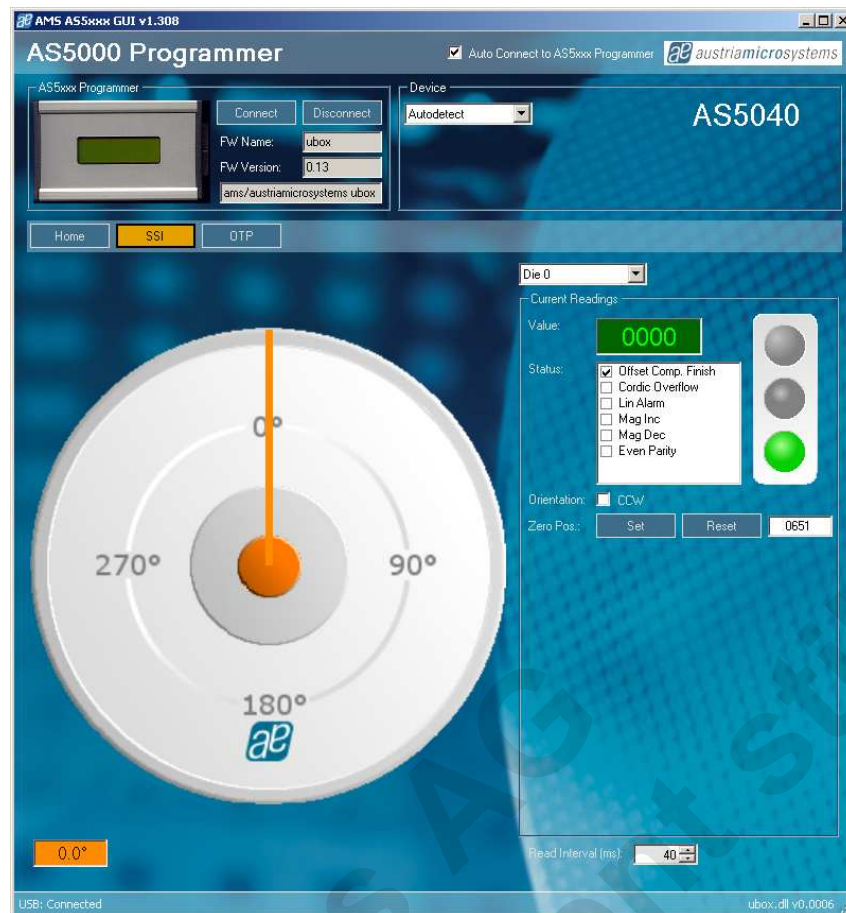
Figure 7: AS5040 SSI tab after Zero Position programming
