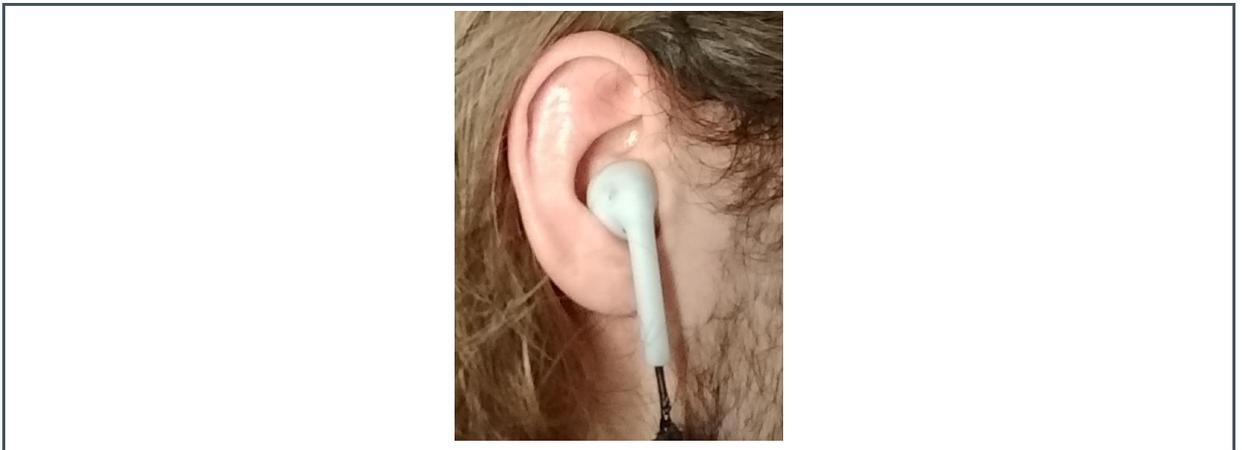
It is very difficult to insert a reference microphone into the human ear, which means that the FB microphone has to be used instead.
