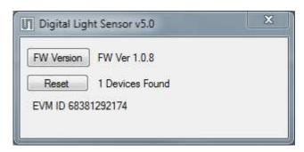
If "No Devices" appears, verify that the daughterboard is connected to the motherboard properly. If "No\_HID" appears, verify the USB cable is connected. A green LED on the motherboard indicates that the USB cable is connected and providing power to the system.
