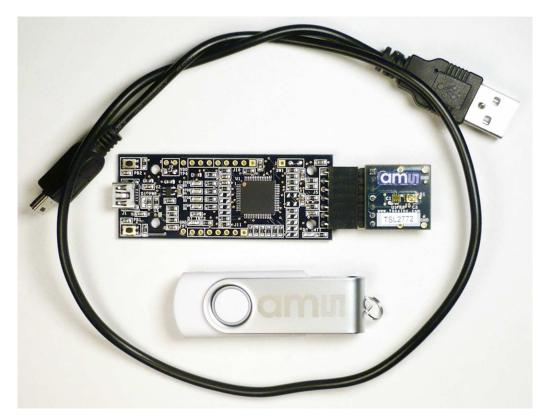
When the USB cable is connected the green LED should light up indicating that power is being received via the USB interface, and the motherboard processor is running. If the green LED does not light up, check the USB cable connections; unplug the USB cable and try again. If the green LED still does not light, check the PC for USB error messages. See the Resources section at the end of this document for additional assistance.
