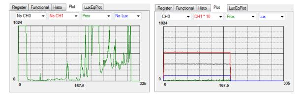
The first plot shows proximity events happening and the second graph shows all outputs for a static system. Multipliers (selected from the list boxes) may be used to scale the display accordingly. On the second plot the Ch1 photodiode is scaled by a factor of 10x relative to the other plotted signals.
