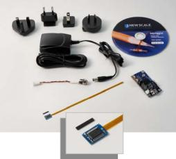
The TRK-1T02-E Evaluation Pack is a fullfeatured development platform for the NSE5310 Position Sensor. The MC-33MB interface card accepts the I<sup>2</sup>C input from one or two NSE5310 sensors, and connects via USB to your PC. Use the New Scale Pathway™ Software to view and collect position information. This development kit provides for easy sensor evaluation and system development.
