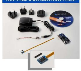
The TRK-1T02-E Evaluation Pack is a full-featured development platform for the NSE5310 Position Sensor. The MC-33MB interface card accepts the I²C input from one or two NSE5310 sensors, and connects via USB to your PC. Use the New Scale Pathway™ Software to view and collect position information. This development kit provides for easy sensor evaluation and system development.
