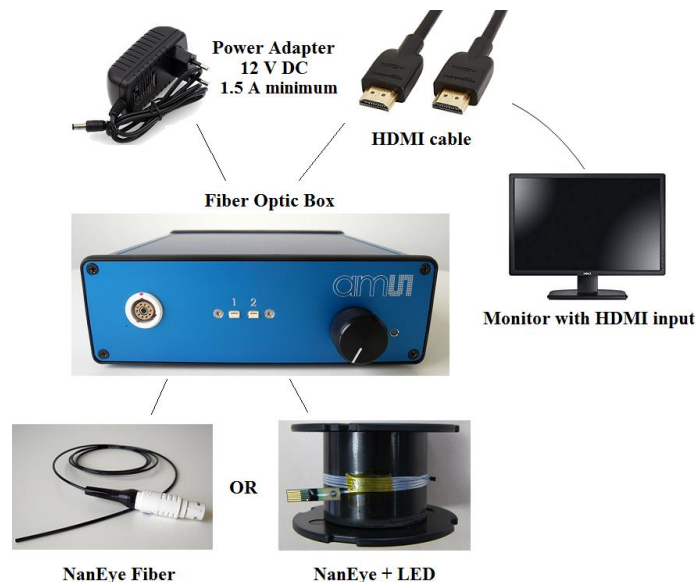
Figure 4: Fiber Optic Box Plug and Play Equipment Connection
