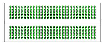
The BB300 breadboard tie-points are connected in 60 vertical columns (the green lines) with 5 connected holes in each. This is the circuit area. When an integrated circuit is plugged into the breadboard, each I.C. pin has a column. There are no horizontal running connections on the BB300.
