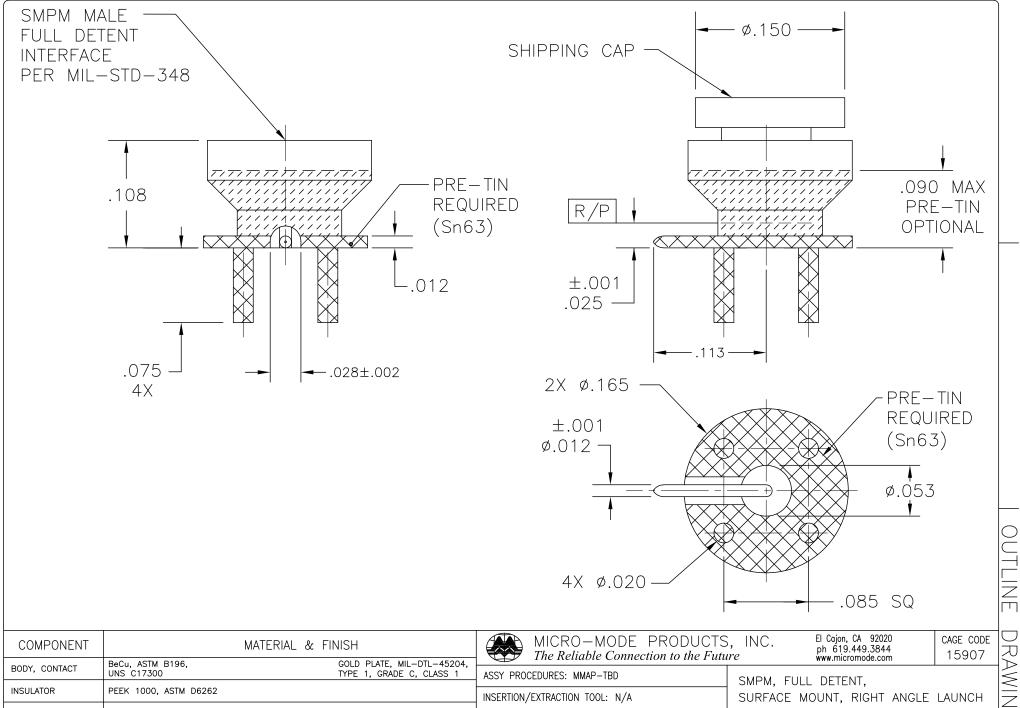
BeCu, ASTM B196, UNS C17300 TYPE 1, GRADE C, CLASS 1 ASSY PROCEDURES: MMAP-TBD SMPM, FULL DETENT, PEEK 1000, ASTM D6262 **INSULATOR** INSERTION/EXTRACTION TOOL: N/A SURFACE MOUNT, RIGHT ANGLE LAUNCH REVISION SOLDER Sn63 (TIN-LEAD) PART NO. MSSP-13761 SHIPPING CAP PTFE TEFLON 11-11-14 . MP SHEET 1 OF 1
