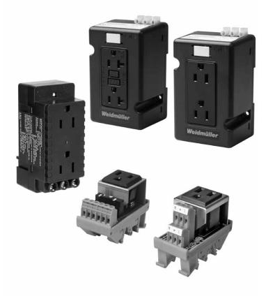
DIN-rail receptacles, 5A, 15A and 20A power outlets, provide a convenient power source for portable computers or test devices for in-the-panel troubleshooting. They mount on standard 35mm DIN-rail. The terminations accept slotted or Phillips screwdrivers. The mounting foot includes a latching lock - slide it open, mount the module on the DIN-rail and slide the lock closed.
