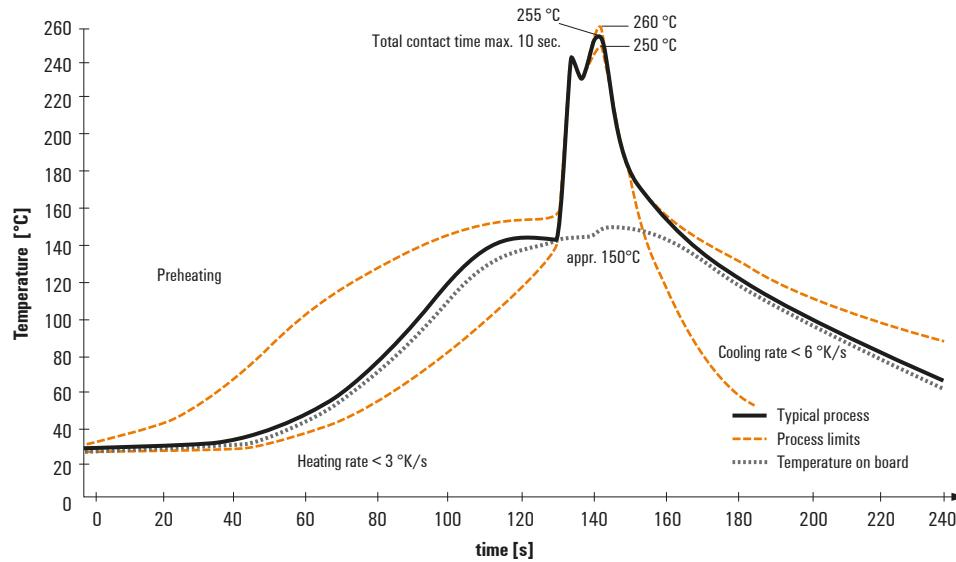
**Wave soldering profiles**
