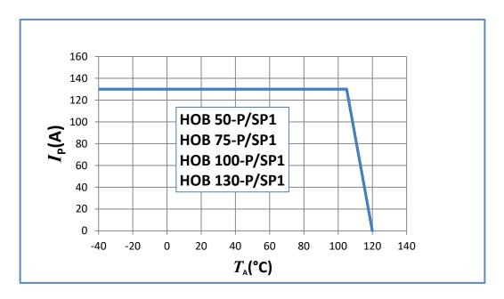
$\underline{Important\ notice}: whatever\ the\ usage\ and/or\ application,\ the\ transducer\ jumper\ temperature\ shall\ not\ go\ above\ the\ maximum\ rating\ of\ 120\ ^{\circ}C\ as\ stated\ in\ page\ 3\ of\ this\ datasheet.$
