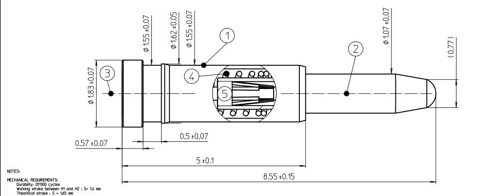
Spring forces (F): Finit= 0.50 N at Hinit= 8.55 mm \* F1= 0.57 N at H1= 8.35 mm \* Fnom= 0.82±0.15 N at Hnom= 7.65 mm
