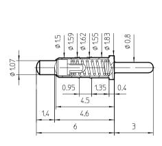
Note: Contact P/N is for basic contact, please add suffix for plating code and, for socket contacts, assembly code.
