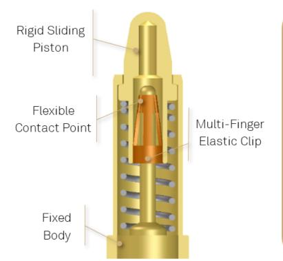
A CLIP establishes a reliable efficient connection between the body and piston. Compliant to: - Shock and vibration up to 2000Hz - Current up to 25A
