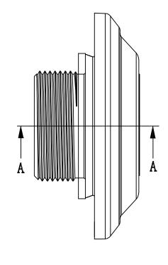
DATE NDTES: 1- BODY MATERIAL - PC (IP67) MEMBRANE MATERIAL - e-PTFE FLAT SEAL WASHER MATERIAL - SILICONE 2- FINISH - BLACK 3- DIMENSIONS ARE INCH [MM] DRAWING FOR REFERENCE WE RESERVE THE RIGHT TO MAKE CHANGES TO DUR STANDARD PRODUCTS. PLEASE CONSULT WITH BUD INDUSTRIES PRIOR TO USING THIS DRAWING FOR DESIGN PURPOSE.
