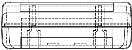
NOTE: MOUNTING BOSSES USE EITHER M2.5 METRIC OR #4 STD. SHEET METAL SCREWS x 3/16" LG. (NOT SUPPLIED)
