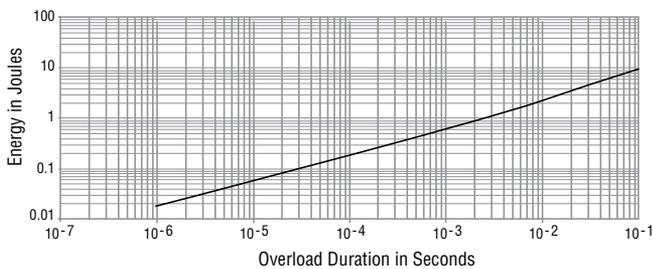
The energy absorbed by the resistor expressed in Joules can be calculated by multiplying the peak power of the pulse in watts times the length of the pulse in seconds.
