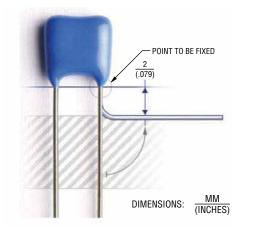
Very often before soldering through-hole components, their leads get bent. It is important not to damage the components during lead bending. Damage most commonly incurred during bending is cracks in epoxy parts, which can lead to increased humidity sensitivity of a component and, consequentially, a shorter lifetime.
