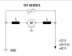
Provides for the elimination of transients and EMI noise in automotive electronics such as engine control, exhaust gas control, safety systems, etc., against disturbances caused by small motors used in automobiles. Most frequently, small motors in an automobile are those used for windscreen wipers, window mechanisms, seat adjustments and automatic door locking.
