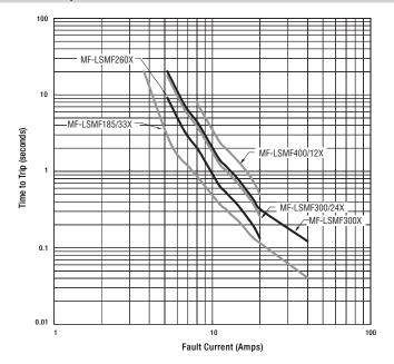
The Time to Trip curves represent typical performance of a device in a simulated application environment. Actual performance in specific customer applications may differ from these values due to the influence of other variables.
