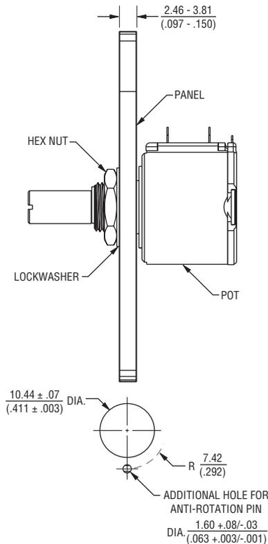
Anti-rotation pin hole is shown at six o'clock position for reference only. The actual location is determined by the customer's application. Refer to the front view of the potentiometer to see the location of the optional A/R pin.
