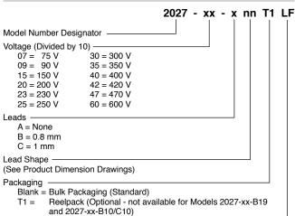
2027-XX-B - 0.8  $\pm$  .04 mm (0.032  $\pm$  0.002 in.) dia. lead wire 2027-XX-C - 1.0  $\pm$  .04 mm (0.039  $\pm$  0.002 in.) dia. lead wire
