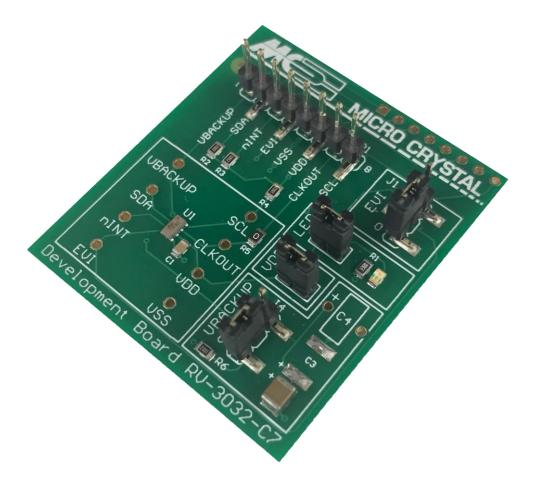
Temperature Compensated RTC Module
