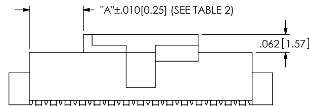
FIG 5 -P: PICK AND PLACE PAD (PAD TO BE ORIENTED AS SHOWN FOR 5-12 POSITION PARTS) (FOR 13-50 POSITION PARTS, PAD MAY BE ORIENTED IN EITHER DIRECTION) (SAME AS FIG 1, DIFFERENT AS SHOWN)
