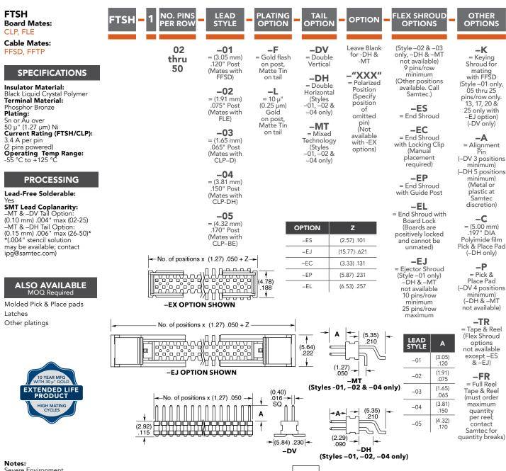
Severe Environment Testing qualified; aligns with MIL-DTL-55302. Visit samtec.com/set
