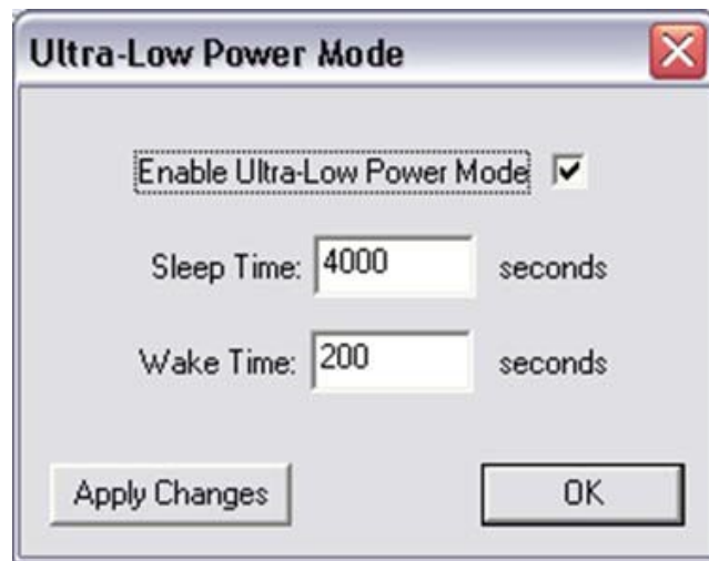
Figure 11 • CSACdemo Ultra-Low Power Mode Configuration Panel
