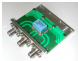
Relay soldered on Test Fixture (4)
